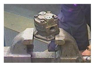
Place the pump in a vise with the drive shaft pointing down. Clamp unit on the sides of the mounting flange. Do not clamp on the pilot diameter as it may damage the seating surface.
