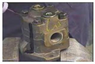
Mark each casting in the assembly with machinist's ink or a prick punch to orient the castings so unit can be reassembled later in the proper position.
