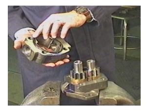
Remove and discard the rubber section seals from the top and the bottom gear housing faces.
