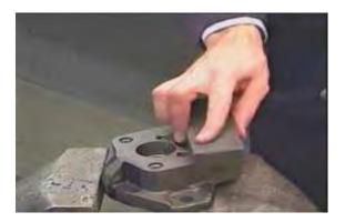
Stone all machined casting surfaces with a medium grit carborundum stone. If the bushings were removed, deburr the bushing bore using a deburring tool. Rinse all parts in a solvent fluid. Air blast all parts and wipe them clean with a clean lint free cloth before starting the assembly.
