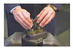
Remove the idler gear and the gear shaft. Keep them together as they are a matched set. Handle with care to avoid damage to the journals, faces, and teeth.
