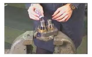
Wipe the gear face surface dry with a clean lint free cloth. Mark the teeth of the gear set at their mesh point with machinist's ink or quick dry marker. This is to index the gear set for proper orientation during reassembly.
