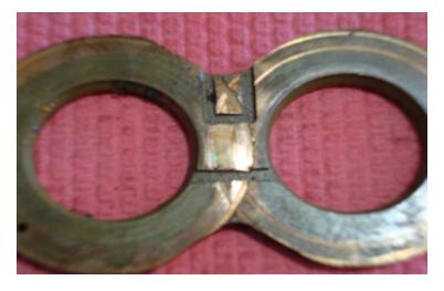
The excessive heat will also result in severe damage to the nylon channel seal and butyl rubber seal on the back of the thrust plate thus propagating further damage to the entire pump and hydraulic system.
