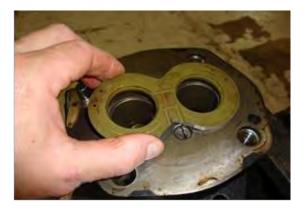
Gently lift off the thrust plate. Be careful not to bend or score the plate and mating surface of the casting. Remove and discard the rubber pocket seals from the back of the thrust plate. NOTE: Pay attention to the orientation of the oil seal and channel on the bottom of the thrust plate.
