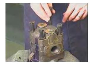
Thread the four cap screws with the washers into the shaft end cover and tighten them in a cross corner pattern. Rotate the gear shaft of the pump with a 6" wrench to make certain here is no binding in the pump.
