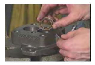
If the shaft seal was removed from the shaft end cover, It should be replaced at this time.
