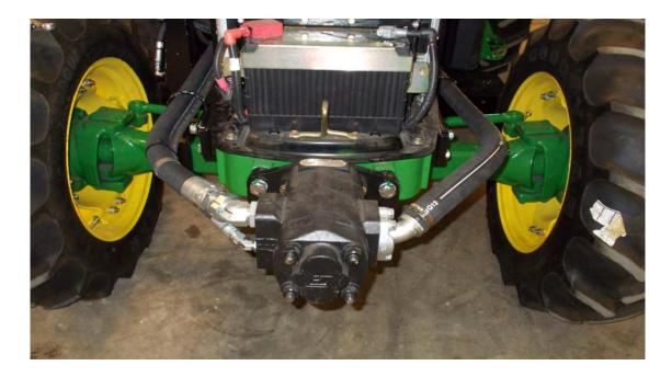
The heart of a hydraulic system is the hydraulic pump. The pump is the component that receives the mechanical energy supplied by the tractor or engine, and converts it to fluid energy with the use of the hydraulic oil.
