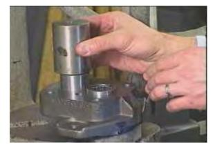
Install the bushings in the shaft end cover and the port end cover. Use an arbor press to press the bushings into the bottom of the bearing bores.
