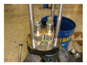
Thread the four cap screws with the washers into the shaft end cover and tighten them in a cross corner pattern. Rotate the gear shaft of the pump with a 6" wrench to make certain here is no binding in the pump.
