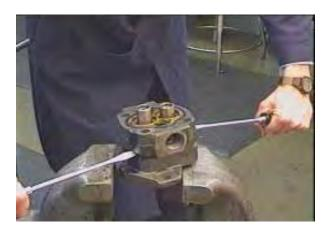
Remove the gear housing subassembly using steps 5.1 through 5.3:
