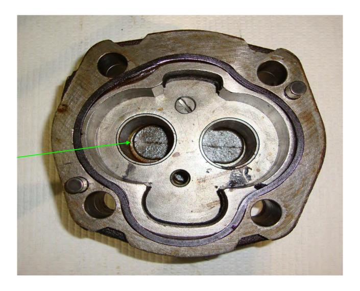
Hydraulic shock loads to the hydraulic system normally result from excessive ground speed while cutting heavy brush or trees and will be displayed as either cracks in the gear pump housing or a broken drive shaft. Shock loads can cause an immediate component failure. Sudden pressure spikes that exceed the pressure rating of the pump can crack the housing at the port location and bolt hole areas of the casting, severely scoring the thrust plate surface, and damage the drive shaft.
