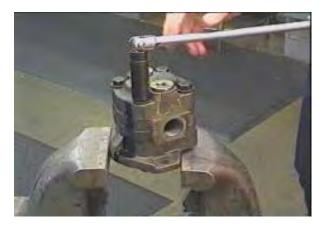
Loosen and remove the four cap screws and washers with a socket and wrench.
