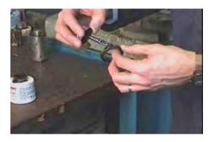
Coat the outside diameter of the lip seal with Permatex Aviation Form-A-Gasket No.3 Non-Hardening Sealant or equivalent.
