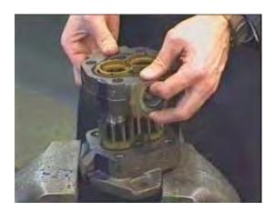
5.2 Lift off the gear housing sub-assembly.
