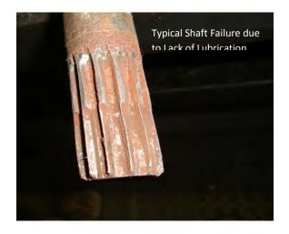
The Drive shaft in the figure displays an example of **fretting corrosion**. Fretting is a condition that occurs between the drive shaft and the drive coupling. These parts are commonly lubricated with a heavy grease/ anti-seize agent. Fretting damage occurs when the grease picks up grit and the small amplitude vibration associated with the normal operation of the mower makes the contaminated grease act like sand paper and produces wear on the shaft.
