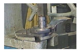
Place the shaft end cover on an arbor press with the pilot facing up. Place the lip seal, with the shoulder of the seal up, at the top of the seal bore. Press the lip seal into the shaft end cover with a lip seal installation bar. The seal should be pressed in so it is flush with the recessed face in the shaft end cover casting.
