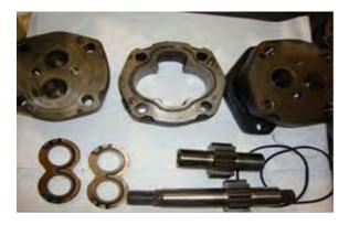
Inspect all the components for wear and replace as required.
