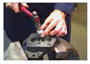
Peen over the check holes in the shaft end cover with a 1½" steel ball and a hammer. This will insure that the checks do not back out of the check holes during operation.
