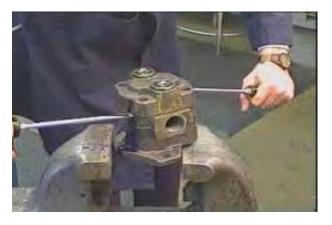
4.2 Place two large flat bladed screwdrivers into the separation notches and pry up the port end cover until loose.
