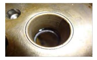
Inspect the bushings for wear. Replace following the next steps if required.
