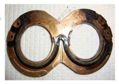
Exposure to excessive heat will also discolor the ends of the gear teeth near the gear face. The high heat causes bluing of the teeth. With continued operation the gear face and thrust plate will start to weld together. Friction generated from continued operation could eventually result in a seized pump.
