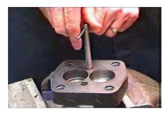
Use a large screw driver or a Check Tool to remove the check valves.
