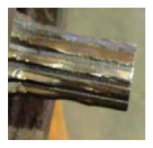
As the wear progresses, the clearance between the parts becomes greater allowing more shaft coupling movement. The wear accelerates until there is not enough engagement to carry the torque load produced during mowing or tree trimming. As a result, the coupler will spin on the shaft and the pump will stop working. To repair, the pump gear set, coupler and shaft will need to be replaced.
