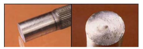
Torsional overload resulting in transverse shear.
