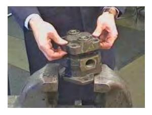
4.3 Lift off the port end cover subassembly.
