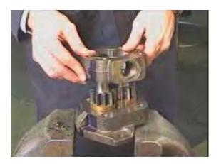
Pace the port end cover over the gear journals. The orientation mark on the port end cover must line up with the mark on the gear housing. Apply pressure to the casting with your hand or tap lightly with a soft faced hammer until the port end cover rests tightly against the gear housing.
