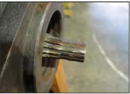
Lack of lubrication of the drive shaft components will result in wear to the splines. High pressure grease or anti seize compound must be applied to all components during installation and replaced at regular intervals throughout the life of the machine.
