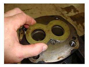
Locate the orientation mark on the gear housing and line it up with the mark on the shaft end cover. Slide the gear housing over the gear set. Make sure that the gear housing rests tightly against the shaft end cover. Be careful not to pinch the section seal. Squirt clean hydraulic oil over the gear shaft and the idler gear to provide initial lubrication when the pump is started.
