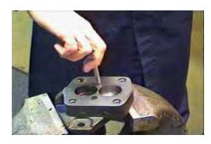
Apply Loctite® No.262 to the threaded check holes in the shaft end casting. Install the checks in the shaft end cover using the check tool
