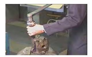
After the cap screws are tightened and you are sure there is no internal binding, tighten the cap screws in a cross corner pattern to a final torque.
