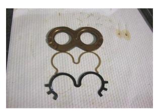
Replace the channel seals in the groove provided on each thrust plate.
