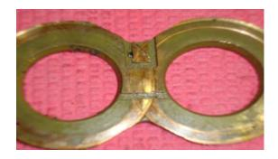
New components provide a smooth, even surface allowing a continuous oil film to exist between the thrust plate and gear face. When these surfaces become scored the oil film dissipates into the grooves interrupting the film. Metal to metal contact occurs, resulting in an increase in friction and heat. The grooved plate surface can also provide an escape route for high pressure oil to go back to the low pressure inlet, resulting in a loss of pumping efficiency.
