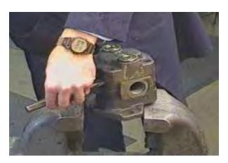
Remove the port end cover subassembly using steps 4.1 through 4.3:
