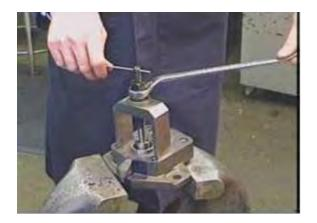
Use a bearing puller to remove the bushings.
